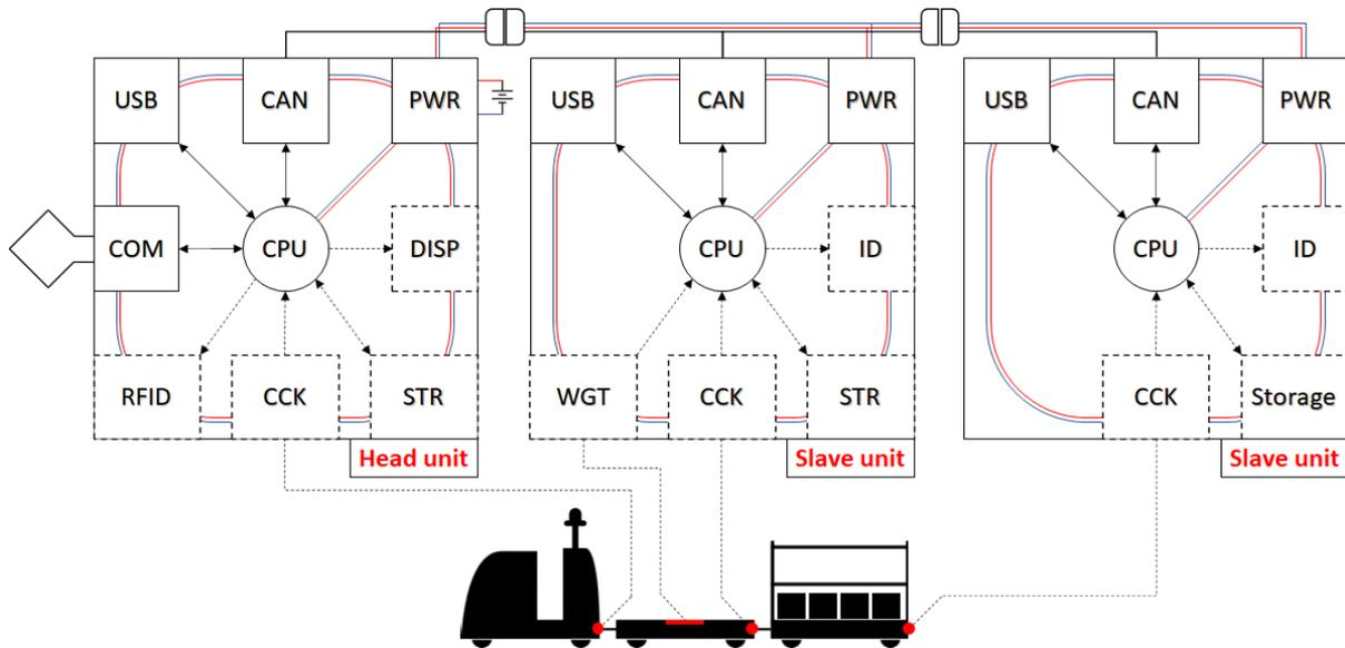
Figure 2: Logical structure of the head- and slave units
