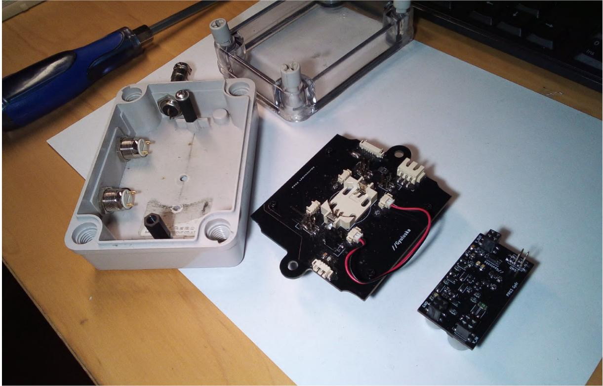
Figure 5: The back side of the master board. To the right is the power module.
