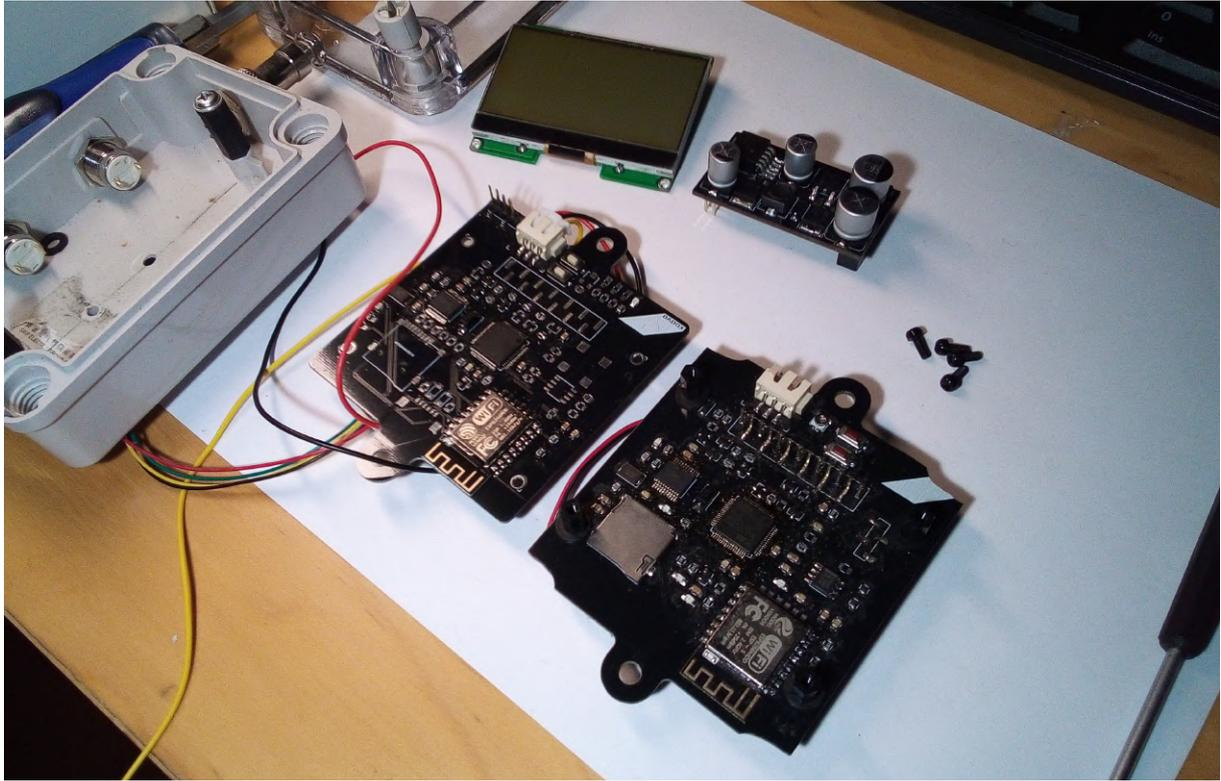
Figure 3: Two master modules. The left one is a newer revision, but the right one has most components soldered in, so that's the one which we'll see in subsequent figures.
