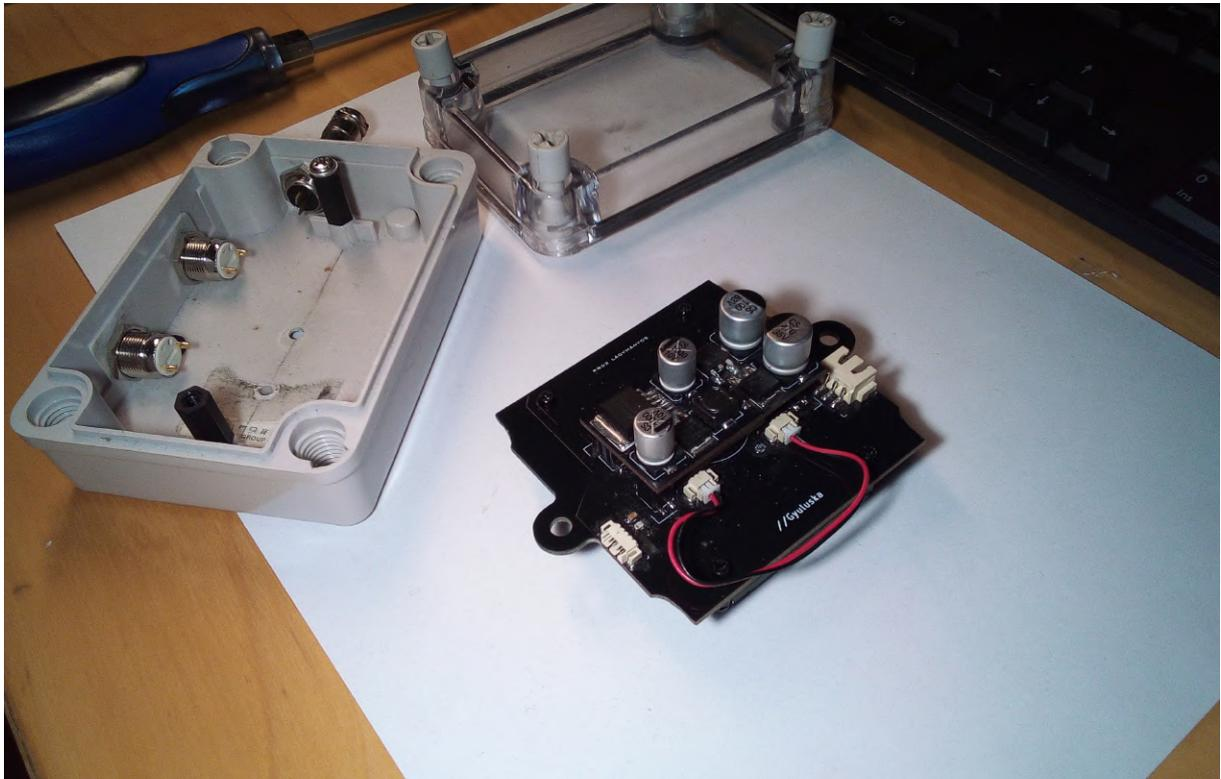
Figure 6: The power module inserted into the master board.
