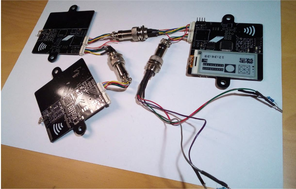
Figure 9: A chain of three slave boards. The rightmost module has an epaper module attached.
