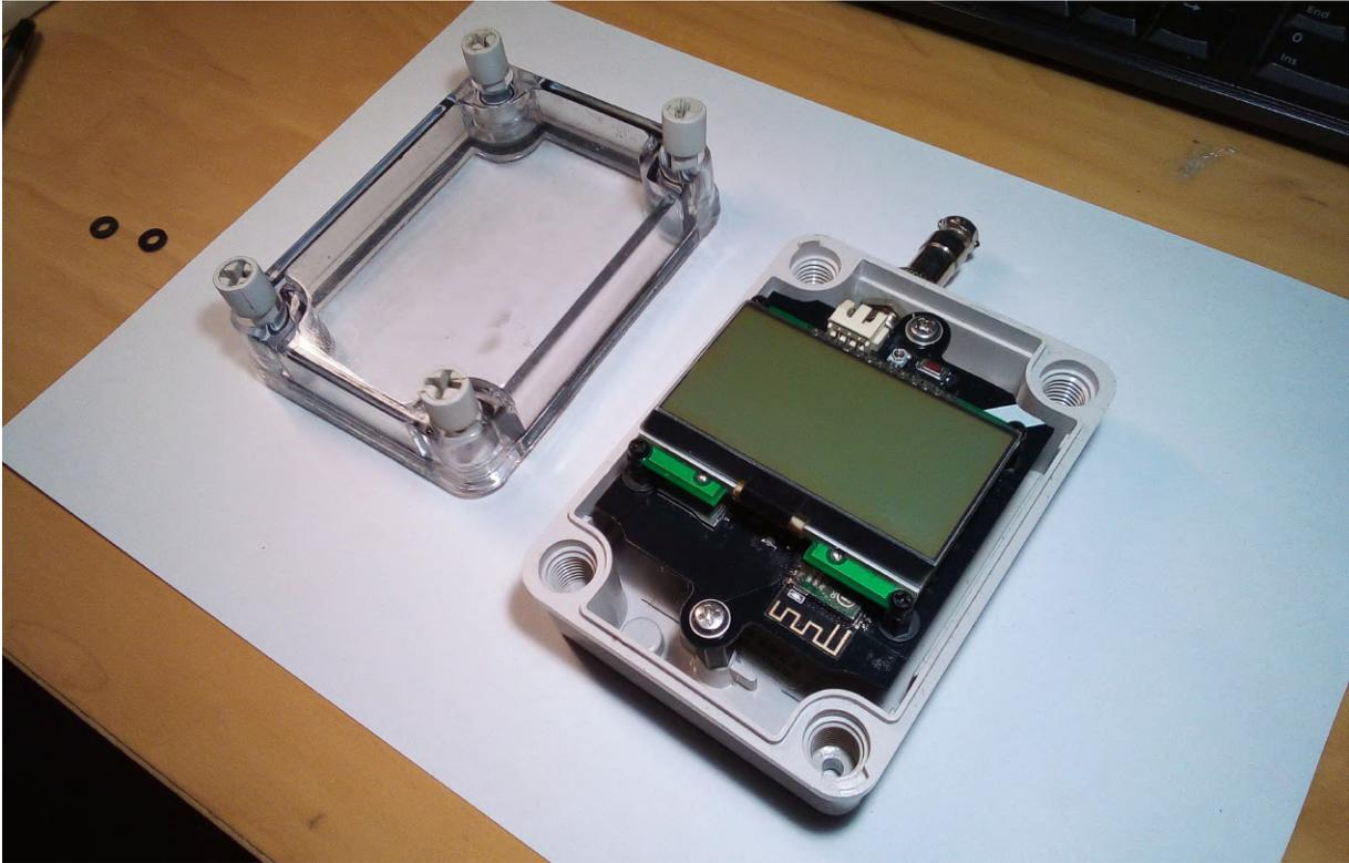
Figure 7: The master assembly fastened in its casing.
