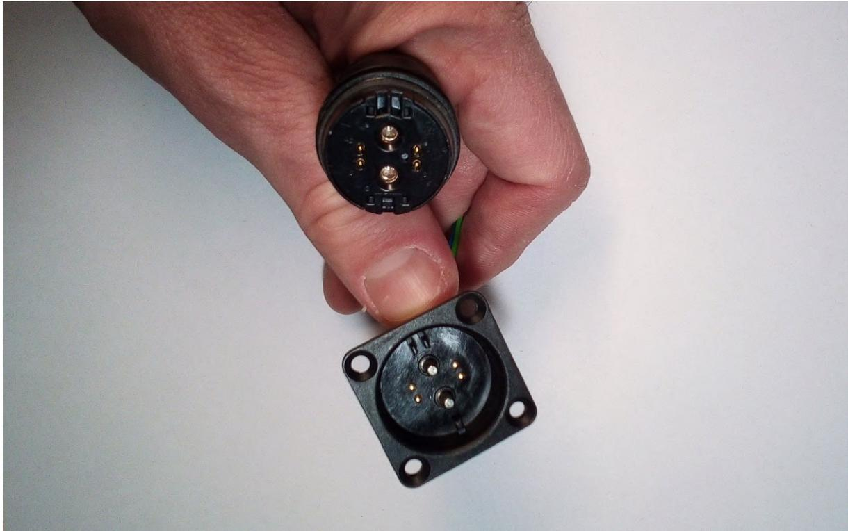
Figure 10: Devices would be interconnected through self-aligning, IP67 water resistant connectors like these from the Rosenberger RoPD line.
